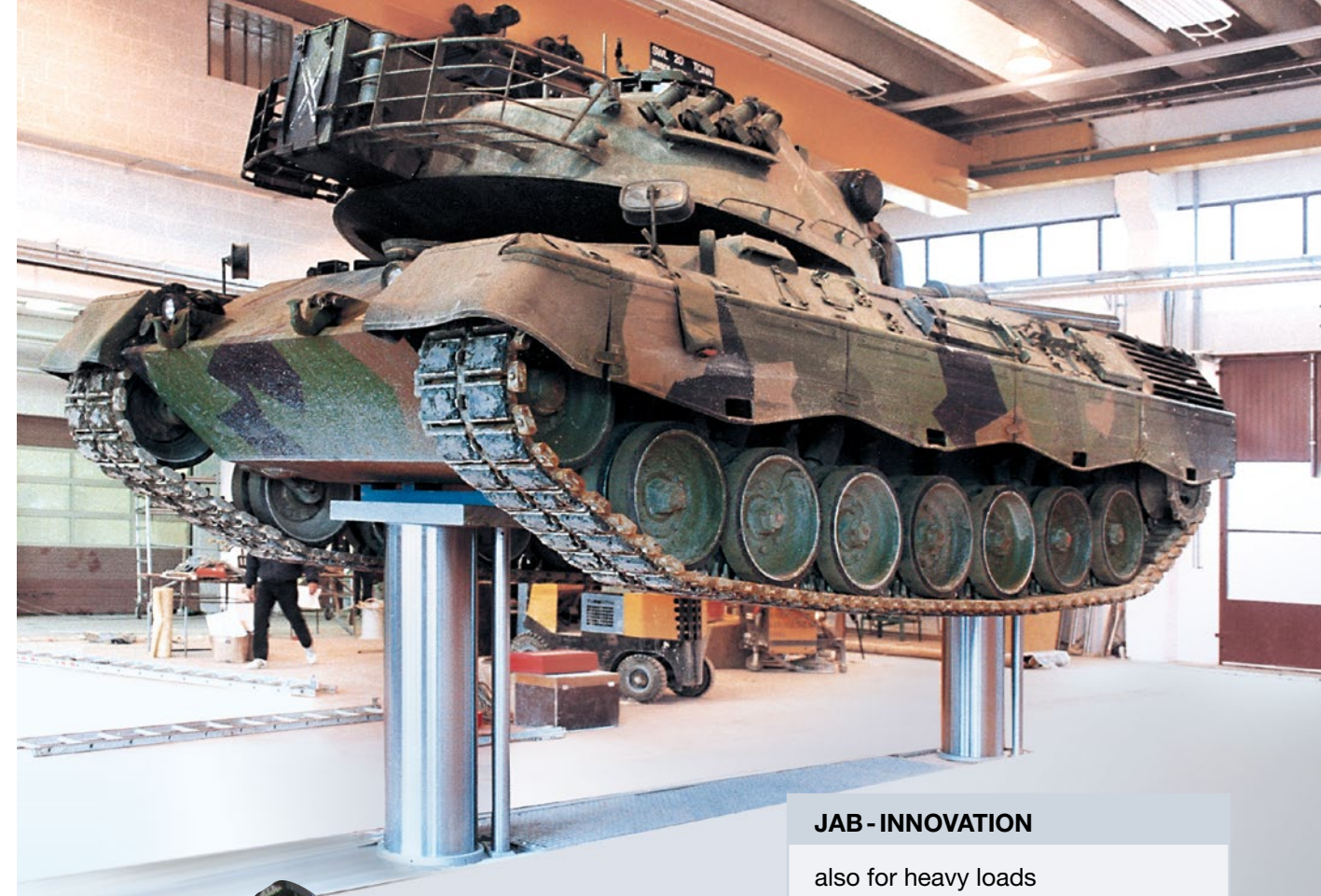
Tanks on a JAB-lift. Lifting capacity 35 t per ram.
