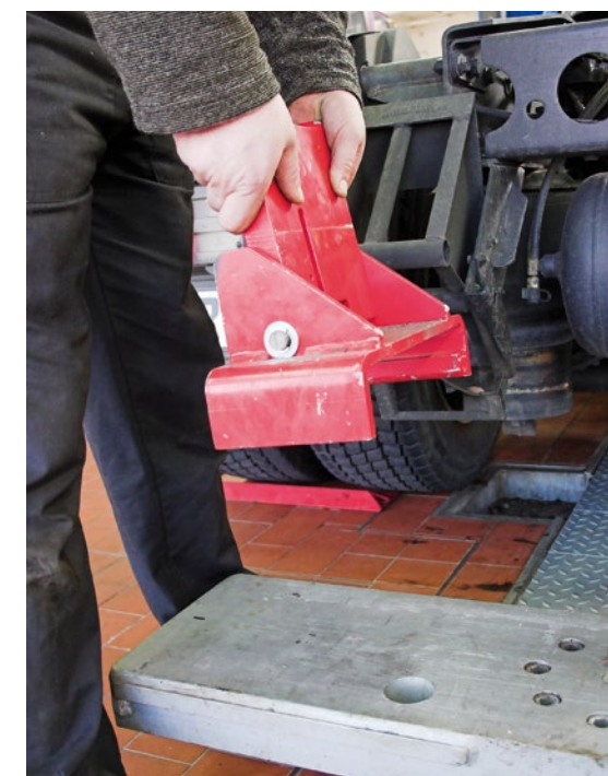
Exchangeable support system for lifting of diverse vehicle types.
