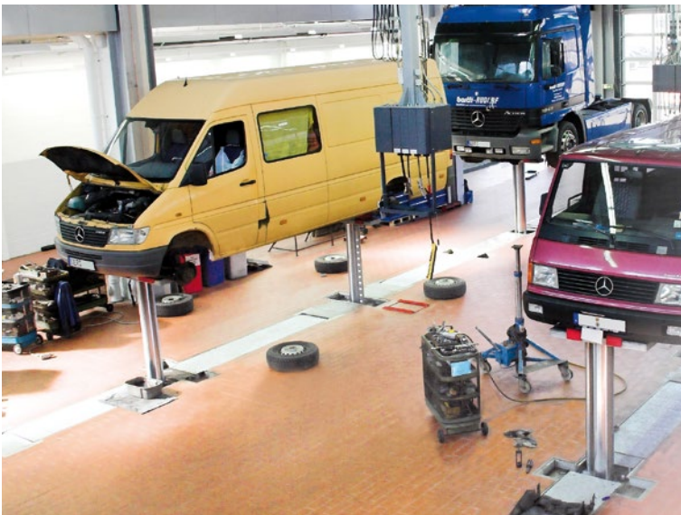
Four-ram-lift HVV, which is used as 2 two-ram-lifts HVZ.
